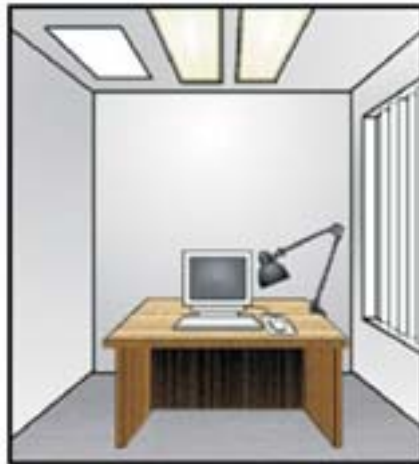
Figure 1 - Blinds are in front of the windows and the monitor is placed at an angle (perpendicular)
